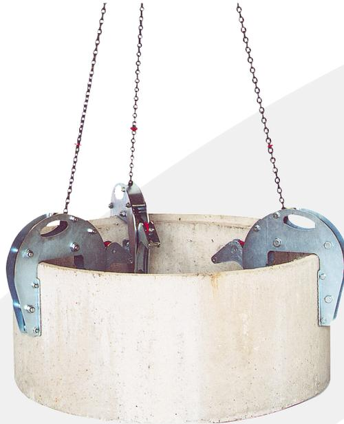
Torsionally rigid light-weight sheet steel construction for the transportation and placement of upright pipes and cones. The shaft ring clamps have been designed in conformance with official labour safety regulations and are equipped with safety locks. (Pre-tensioned springs).
