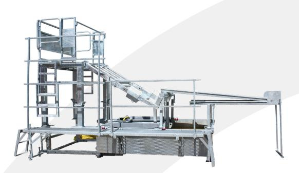
The 3022 Waste water sedimentation tank has a triple chamber system ideal for separating waste water from the solid particles created during the washout of concrete skips. The waste water can be "recycled" for cleaning of a second unit or chemically treated using the 3024 water treatment system for conversion into pure water ready for disposal.
