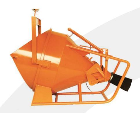
The 1018 has been designed by Eichinger to meet the specific needs of pouring concrete into formwork in a cost effective and efficient way. With the delivery hose attached to the gate of the skip users can direct the flowing concrete with ease. The 1018 makes life easier for the users by 'laying down for filling' as well as the levered gate mechanism for quick, high volume pours increasing user confidence.
