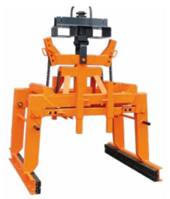
Mechanical gripper for the safe and reliable handling of bulk building materials; with pouches for forklift prongs with manual turner and a suspension eyelet for crane operation; with exchangeable rubber clamping jaws and fully automatic change-over from full to empty.
