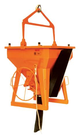
Universal concrete skip, square shape with rounded corners, usable with straight or lateral outlet with moveable flow control chute and pullwire, or with straight outlet with hose coupling and pull-wire.
