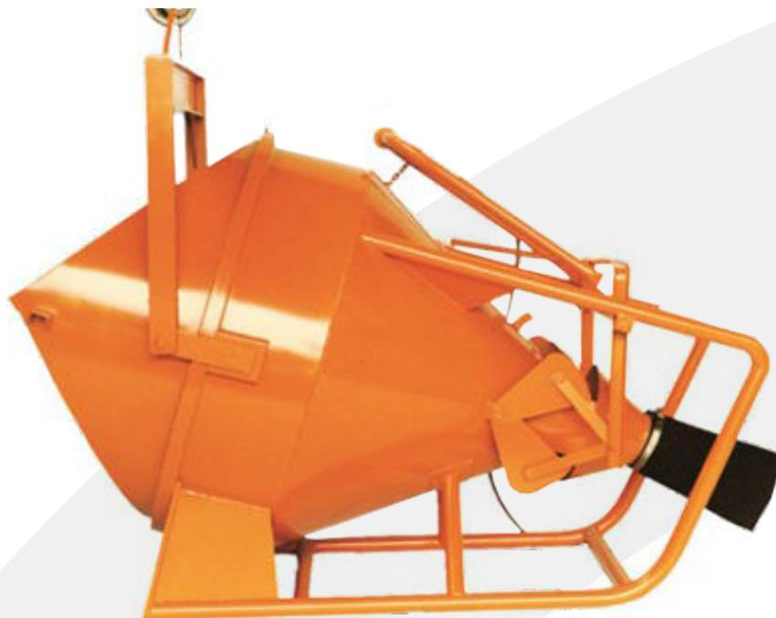
The 1018 has been designed by Eichinger to meet the specific needs of pouring concrete into formwork in a cost effective and efficient way. With the delivery hose attached to the gate of the skip users can direct the flowing concrete with ease. The 1018 makes life easier for the users by 'laying down for filling' as well as the levered gate mechanism for quick, high volume pours increasing user confidence.
